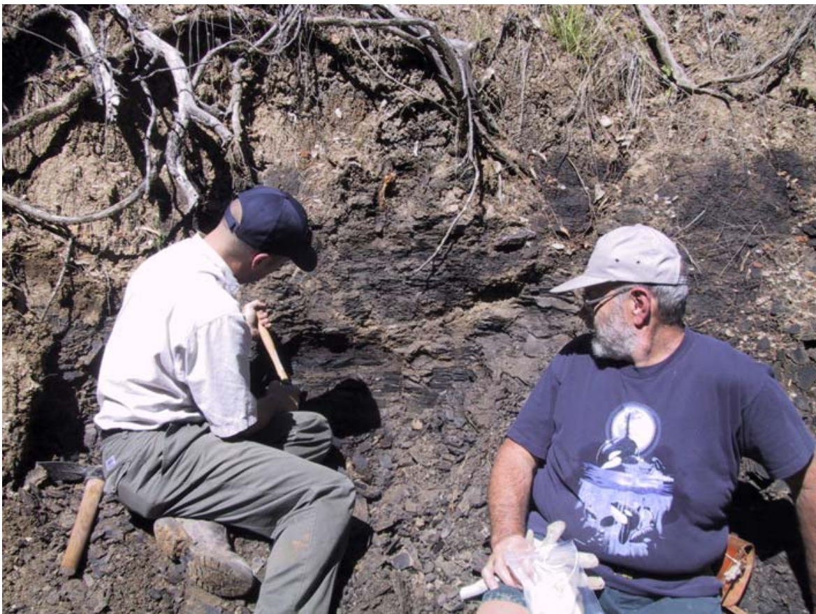
Fig. 2. Rob Creaser (left) and Bob Nicoll (right) collecting organic-rich mudstones for Re-Os dating.
