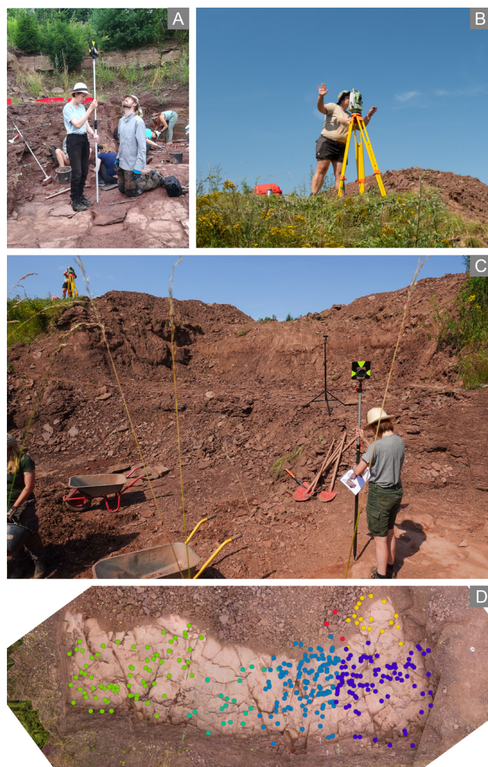
Fig. 5. Total station data acquisition. A-C. Measuring a findspot via total station. A. One person holds the reflector staff, that is placed on a measuring target on the topside of the find, upright; B. the other person targets the centre of the prism via total station and C. pushes a button so that the targeted point is measured. D. The measured points can be visualised in a geographic information system software: all findspots in the northwestern excavation area of the dig in 2022 are plotted in an orthophoto generated on the last excavation day. The different colours represent the six sectors the respective finds were exposed in. Photos courtesy of Anastasia Voloshina (B-C) and Peter Rohde (D).
